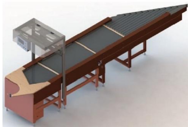
Dynamic Weighing Induction Station
