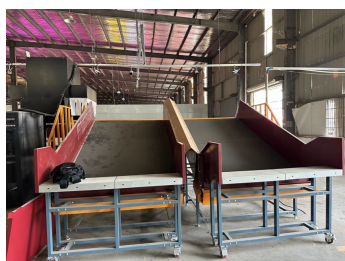
Three-Section Induction Station
